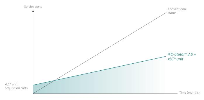
Reducing service costs (spare part and labour costs): A comparison of a NEMO® pump with conventional stator and a NEMO® BY045 with iFD-Stator® 2.0 + xLC® unit clearly shows the enormous savings and rapid amortisation of the xLC® unit's acquisition costs.
